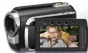
2004: The world’s first Camcorder with built-in hard disk drive as the recording medium. Compact and lightweight, it enables long-time recording.
